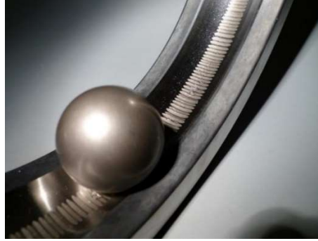
Figure 2. 5. Bearing exposed to bearing current. Bearing race track damaged due to EDM current [49]
